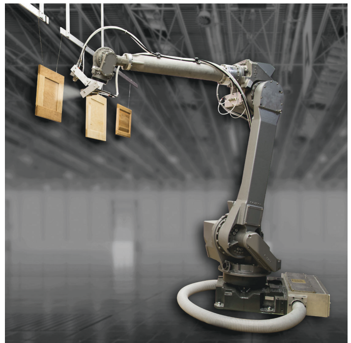
P-350iA/45 coating cabinet doors of various sizes
